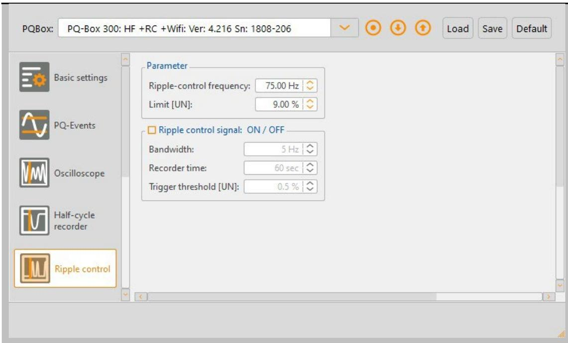
In the ripple control signal frequency field any frequency can be entered in the range from 100 Hz to 3,750 Hz. This frequency now will be permanently recorded as a maximum value of 200ms interval in the cyclic data.
