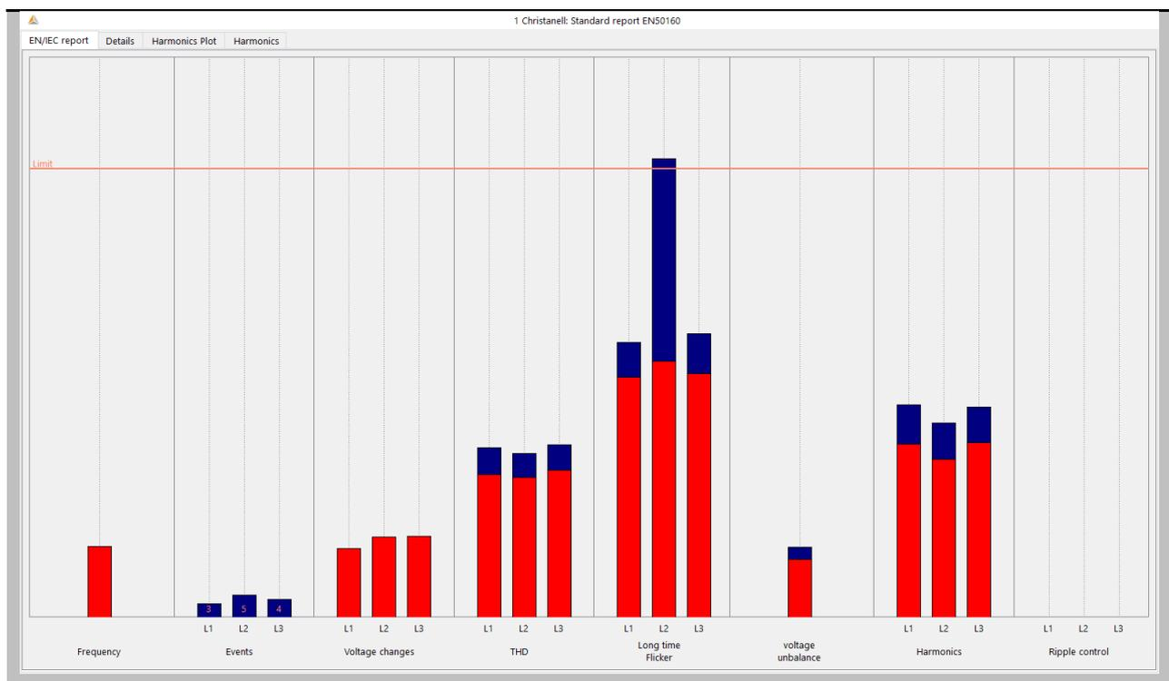
The bars show in a very easy to read form the 95% measured value in red color and the highest occurred measured value "100% value" in blue colour.
