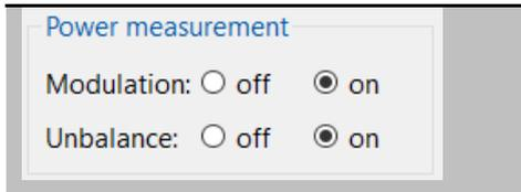
Power calculation with calculation of the unbalance reactive power and the modulation reactive power is the factory setting of the device.
