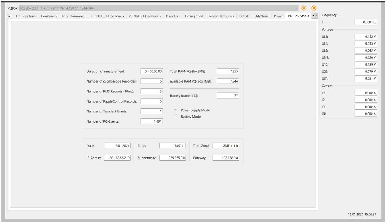
The screenshot displays the 'PQ-Box Status' interface for a PQ-Box 200. The interface includes a navigation menu at the top with options like 'FFT Spectrum', 'Harmonics', 'Inter-Harmonics', '2 - 9 kHz U-Harmonics', '2 - 9 kHz I-Harmonics', 'Direction', 'Timing Chart', 'Power Harmonics', 'Details', 'U/I/Phase', 'Power', and 'PQ-Box Status'. The main content area shows the following data:
