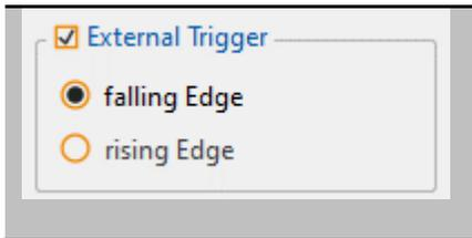
A digital input for an external trigger signal is available via two 4 mm sockets. This input starts the oscilloscope and/or half-period RMS recorder.
