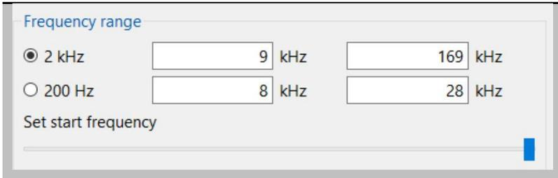
The start frequency of the 2 kHz or 200 Hz frequency bands can be changed with the "Set start value" slider.
