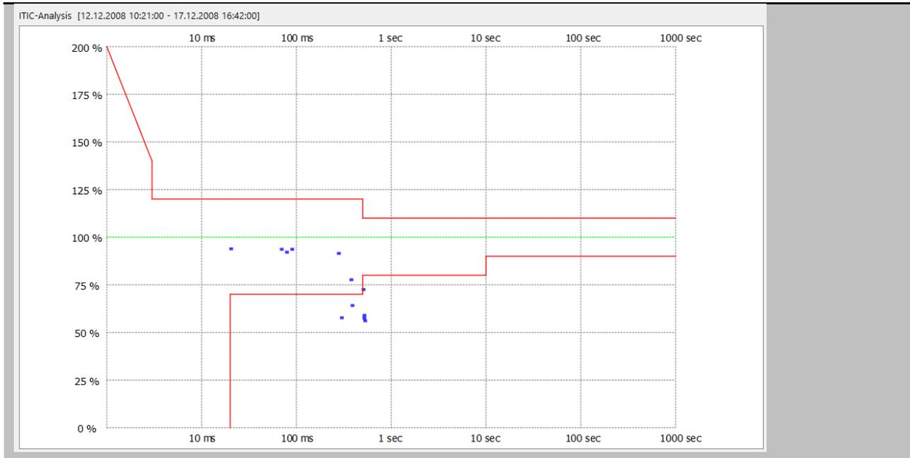
In addition to the ITIC graphic, the "PQ events" card contains an event table "UNIPED statistics" for all voltage dips and overvoltages.
