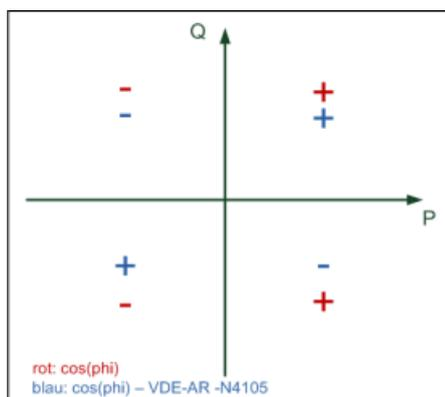
On device display and in online measurement data, the standard cos phi (version a) is shown.
