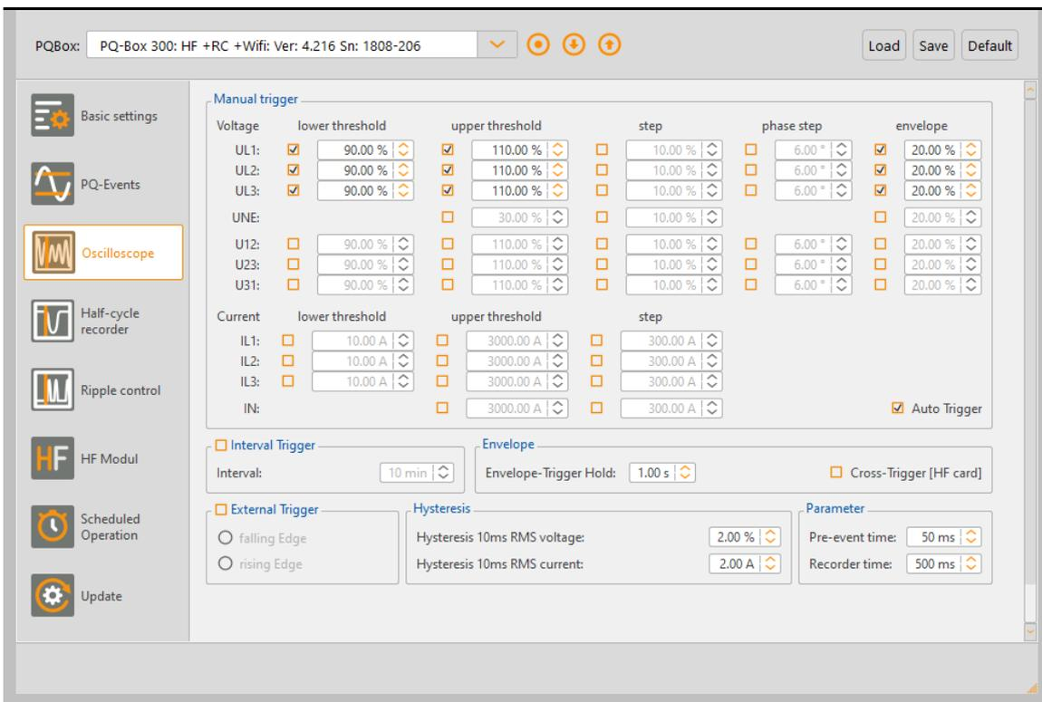
The **recording length** is the total recording time for the oscilloscope record in milliseconds. The "prehistory" is defined as the time recorded before the event occurred. The length of the oscilloscope record, as well as the prehistory can be freely changed from 20ms to 4000 ms
