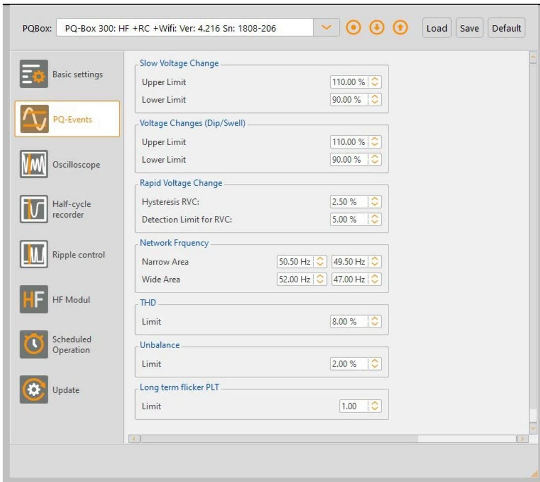
The limit values for PQ events can be set independently of the statistical evaluation of the measurement data. If one of the limit values is violated, this event is saved as a PQ event and later displayed in the software as a list or ITIC diagram.
