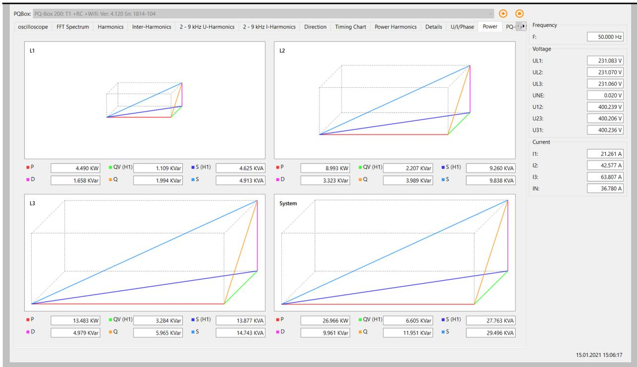
The graph shows the individual power values once for the total RMS value and once for the fundamental vibration values.
