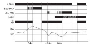
**Untercurrent monitoring (UNDER, UNDER+Latch)**When the supply voltage U is applied, the output relay R switches into on-position, if the measured current is beyond the Min-value. When the measured current falls below the Min-value, the output relay R switches into off-position after the interval of the tripping delay (Delay) has expired.
