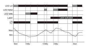
Measuring range 100mA, supply voltage 230V AC
