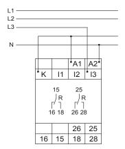
Measuring range 1A, supply voltage 230V AC
