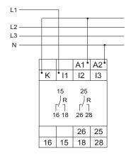
Measuring range 10A, supply voltage 230V AC
