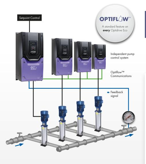
Fully automatic, self-redundant, energy efficient control for boosters with the highest level of overall system protection.
