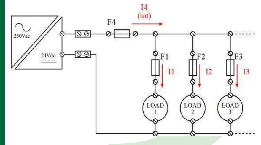
F1, 2, 3 are protections matched with each single load current F4 main protection has to be matched with total current so it requires higher switch-off current than F1, F2, F3
