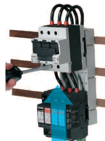
1. Place the component on the top mounting rail and connect 2. Place the component on the lower mounting rail. Position the lower mounting rail to suit component and then connect.
