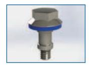
Customized convex blind nut with under head special design for antiloss purpose equipped with gasket. Threaded path length foreseen for guarantee a certain mechanical stop, to avoid excessive gasket compression.
